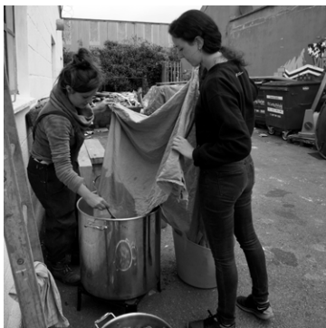
3 Gradually dipping the cloth into the water dye bath
